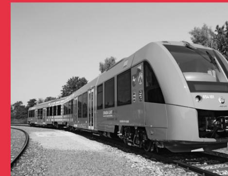
Alstom, electric fuel cell hydrogen train
